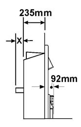
**Dimension X** is 50mm. This can be deleted when installing into a pre-cast or clay flue block system.
