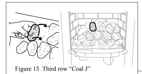
19. Hold coal 'J' upright with the arrow pointing to the top. Locate coal 'J' as shown in figure 15
