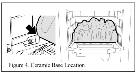
1. Place the ceramic base coal in the burner compartment. The bottom rear face of the coal should rest on the angled ledges at the back of the burner compartment. The bottom front edges of the coal base should locate against the left and right hand side brackets. (See figure 4).
